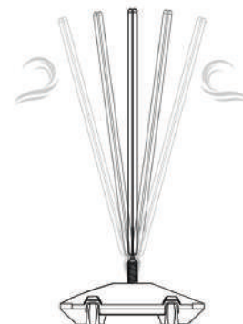
Heavy-duty coil springs resist strong winds and return the sign to an upright position
